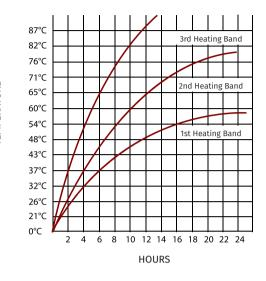
When only 1 heating band is used, it should be installed in the lower section of the drum for best performance.
